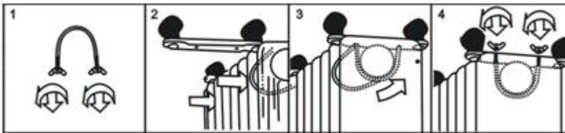
1. Place the radiator body upside-down on a scratch-free location, make sure it is stable and will not fall.
